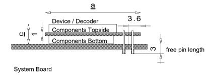
Fig. 1: Arrangement of the decoder on the system board, dimensions according to table 2
